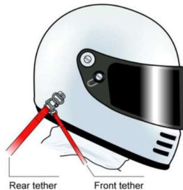
Figure3 Identification of a Hybrid device's tethers
