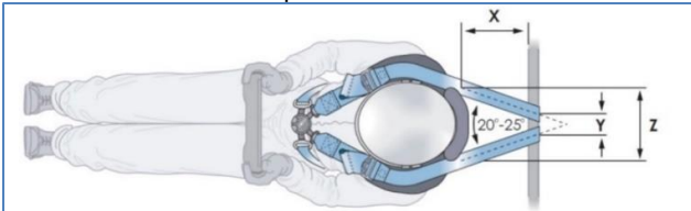
Figure 12 Position of shoulder belt anchorage points to achieve desired belt angle (plan view)
